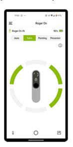
The Roger On mic is small, just under 4 inches long. It can be worn on a lanyard around the speaker's neck (Speaker mode), or held in your hand and pointed at the speaker (Pointing mode), or placed on a table to hear all around (Table mode). In Table mode, a Roger On can listen in six different directions, while in the other two modes it listens only in the direction it is pointed. It adjusts its directionality and sensitivity according to which mode is being used.
